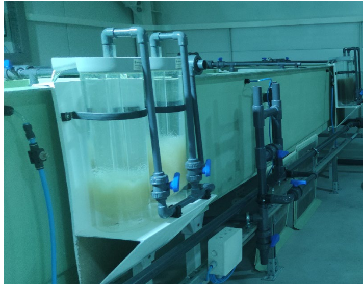
Figure 2. Pikeperch egg incubation in a recirculation aquaculture system Source: Author's own personal archive
